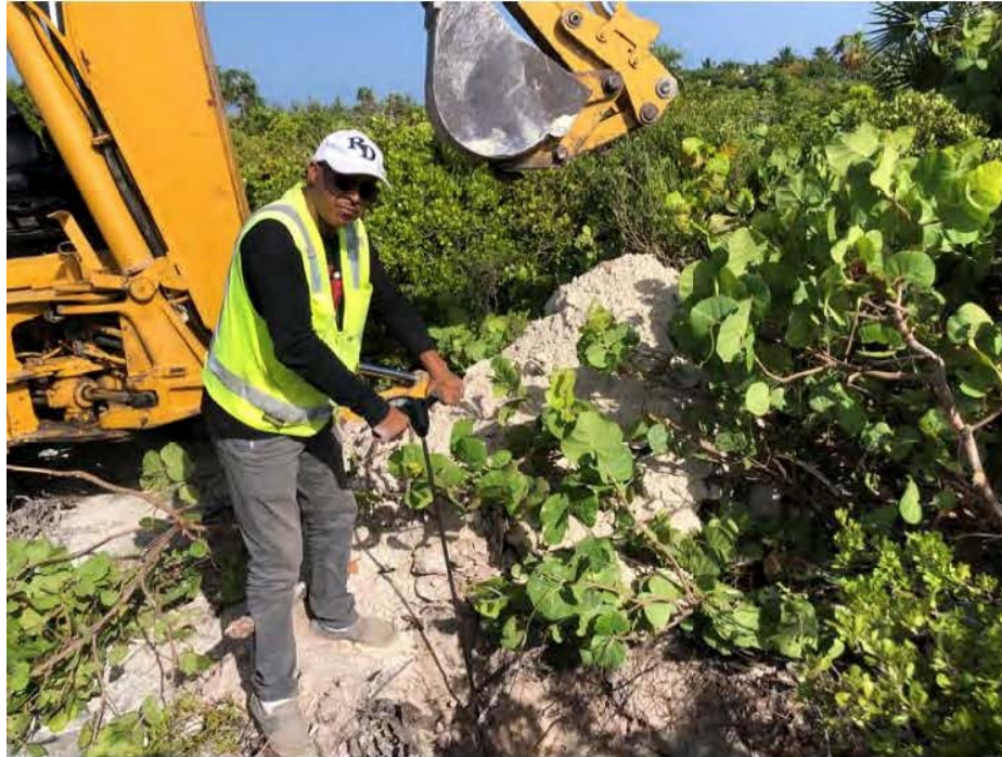
Photo 2-24. Trail 60-degree cone tip resistance at- 2ft is 12kg/cm 2 . Oolitic white sandstone uniformly underlines (Tolleson, 2019)
