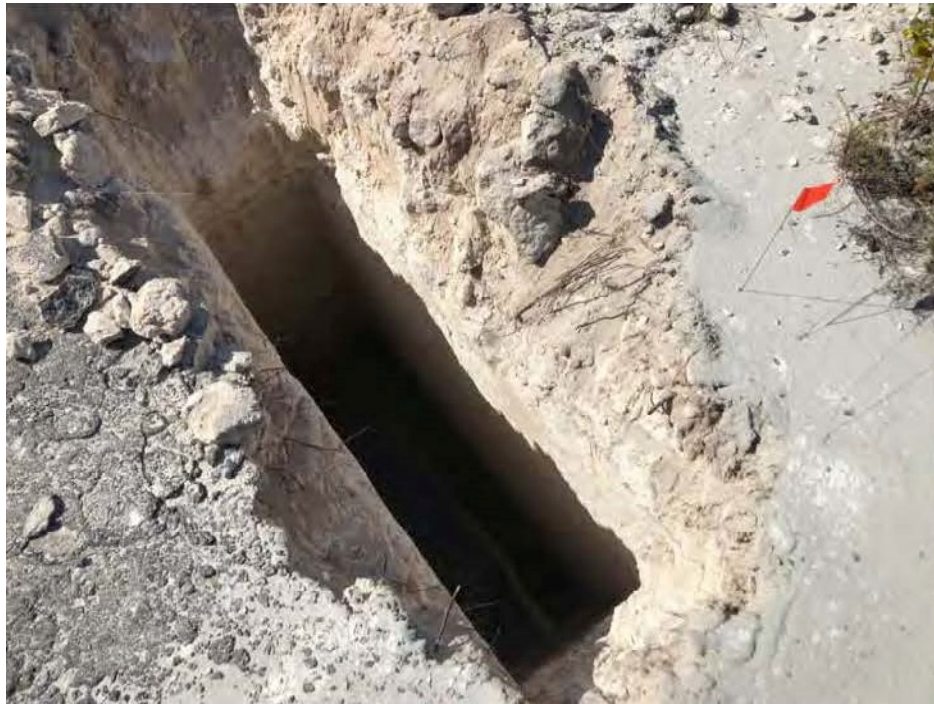
Photo 2-25. Trial pit excavation. Note Clean open pit. Excellent bearing capacity. (Tolleson, 2019)
