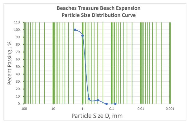
Figure 11. Grain Size Distribution Curve
