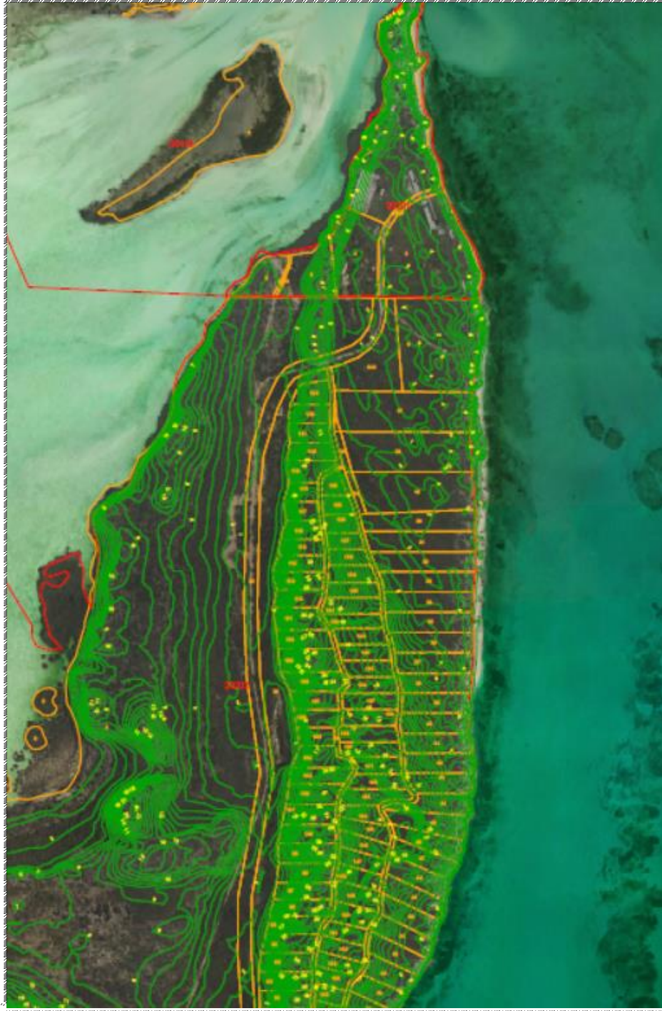
Figure 21: Contour maps that were digitized to produce topography points up to +4msl
