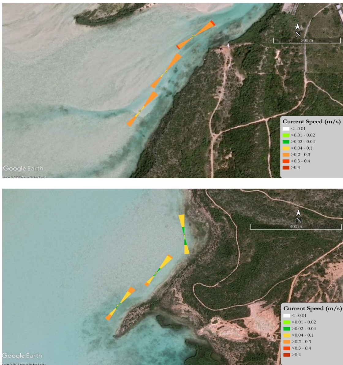
Figure 59: Current speeds and directions (going to) over the 24-day period at three different locations in the nearshore of the project site at the location of both the proposed Northern (Top) and Southern (Bottom) channel entrances.
