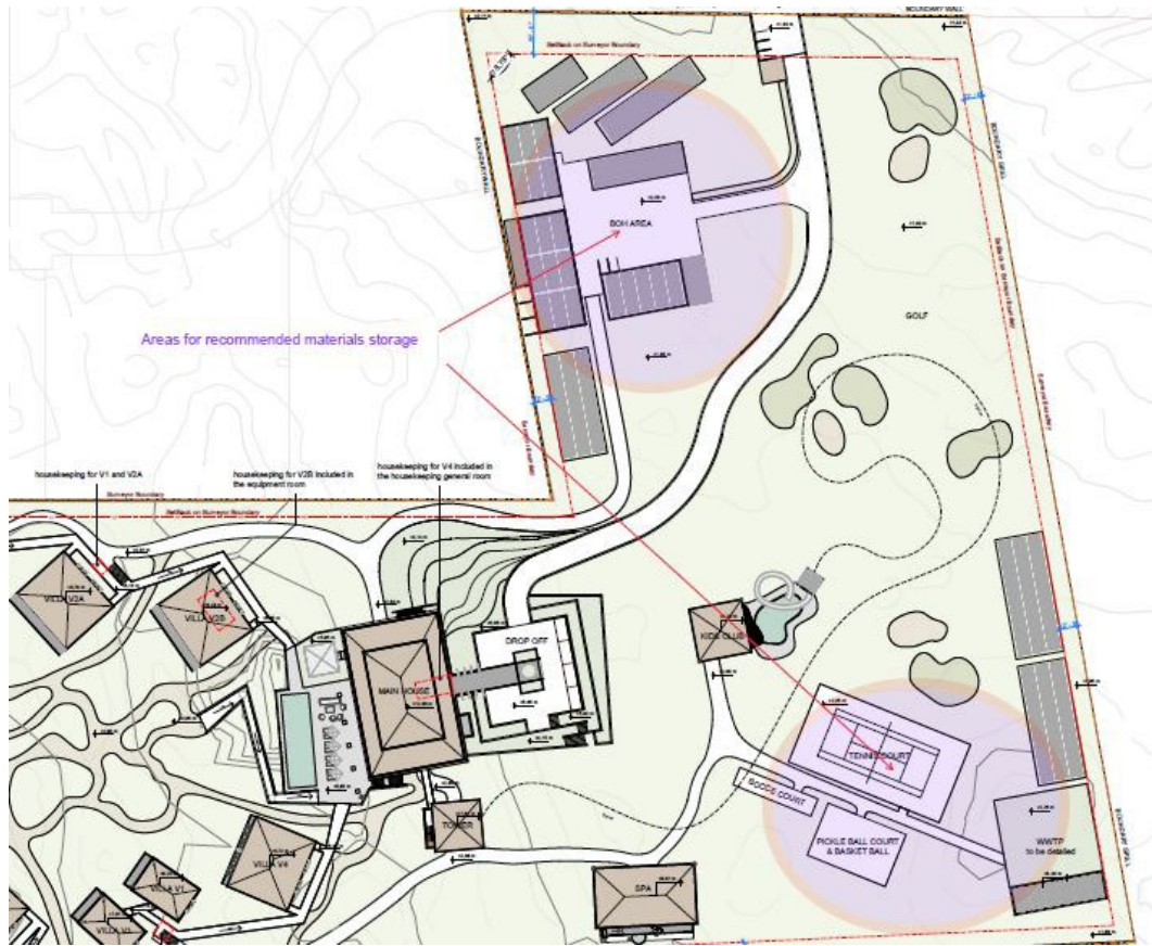
Figure 51 - Areas for recommended materials storage
