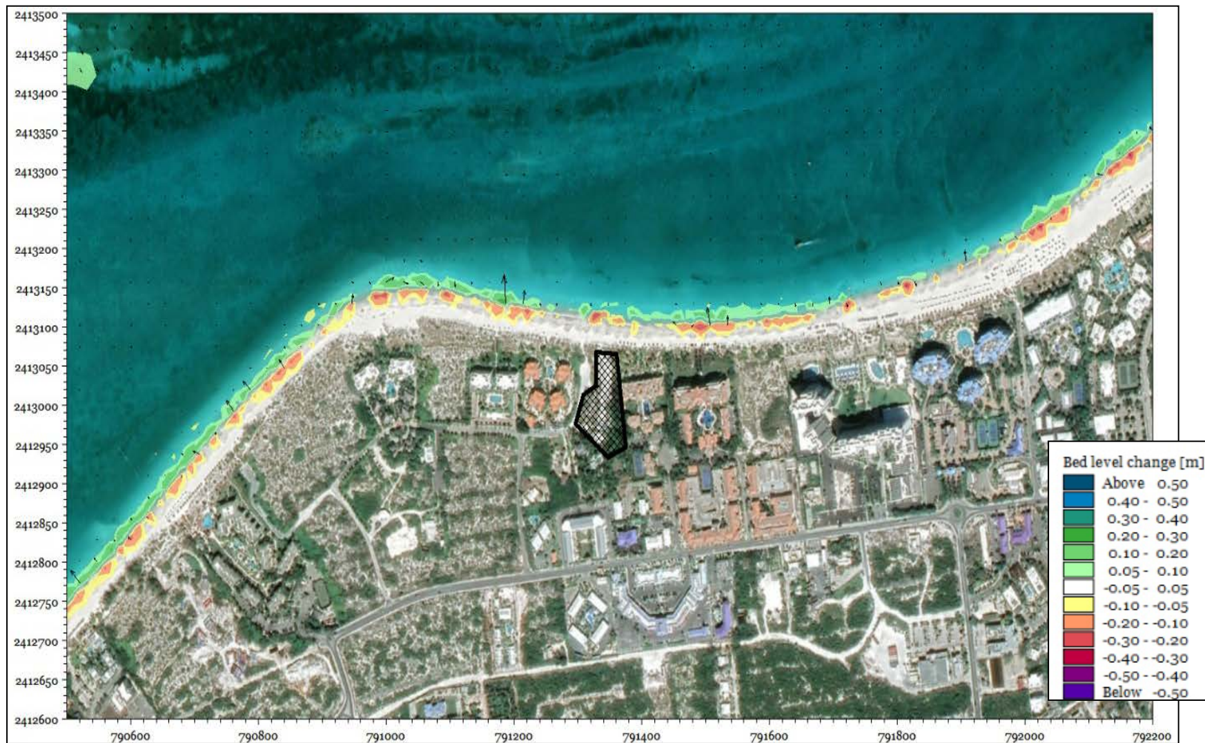
Figure 38.0: Swell event simulation results for bed level change at the last timestep
