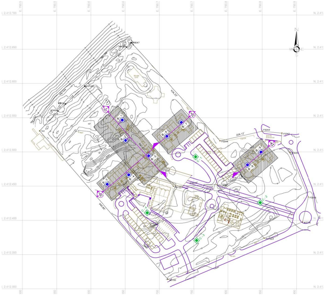
Figure 2-4 Existing Ground Conditions
